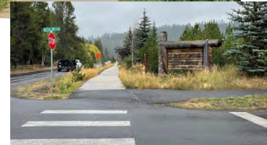
Pathway crossings of streets require detectable warnings and other curb ramps features.
